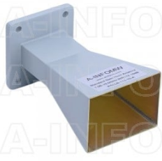
LB-112-10-A Standard Gain Horn Antenna 7.05-10GHz 10dB Gain Rectangular Waveguide Interface
